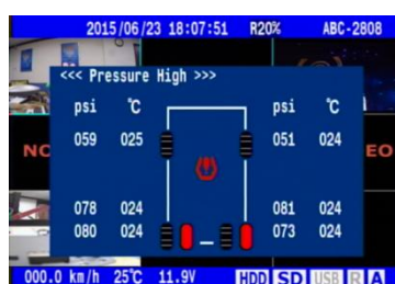
HIGH pressure Alarm
