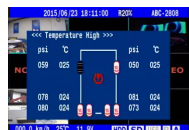
Over temperature Alarm
